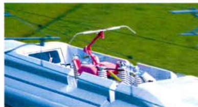
検測・集電兼用パンタグラフ Pantograph for inspection and current collection
